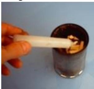
The burner can be lit with a candle, dripping wax onto the topmost layer.
