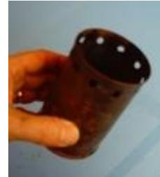
Put the smaller can into the larger one. This arrangement allows wood gas to circulate down through the bottom of the small inner can and up the inside of the side wall cavity mixing with air as it goes. It burns when it re-enters the small can near the top.
