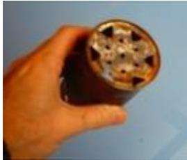
The smaller can has a series of holes pierced in the bottom and 6mm holes drilled in the side near the top and in the bottom. One way to avoid bending the inner can during drilling is to use a round wooden mandrel clamped in a bench vice to hold the can. Drill through into the mandrel then rotate the tin for the next hole.
