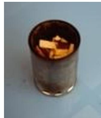
The fuel needs to be from a sustainable source: e.g. hedge trimmings, cut into small wood chips. These should come up to the level of the holes. 57-70g wood chip is sufficient to boil 1 pint (475g) water.
